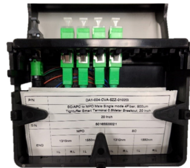
Test record found behind removable cover
